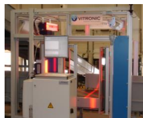
Example for fully automatic data acquisition: codes are read without manual intervention by an operator
