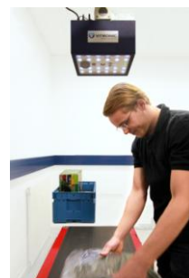
Example for semi-automatic data acquisition: codes are read while the article is moved underneath the camera
