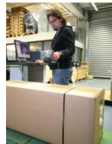
Example for manual data acquisition: the code is identified with a hand-held scanner
