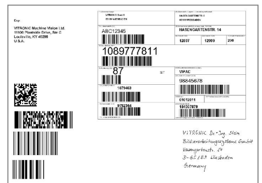
Cameras produce an image and also scan all barcodes, 2D-codes and plain writing (OCR) therein.
